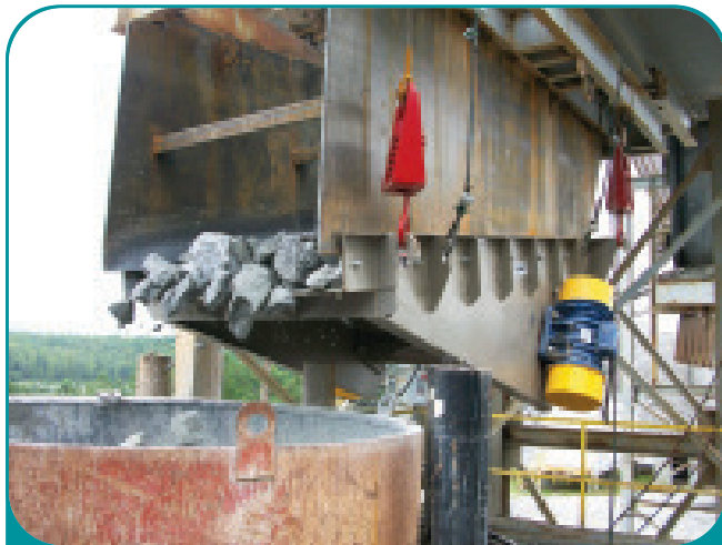
Electric Rotary Vibrators in Primary Feeder Application
