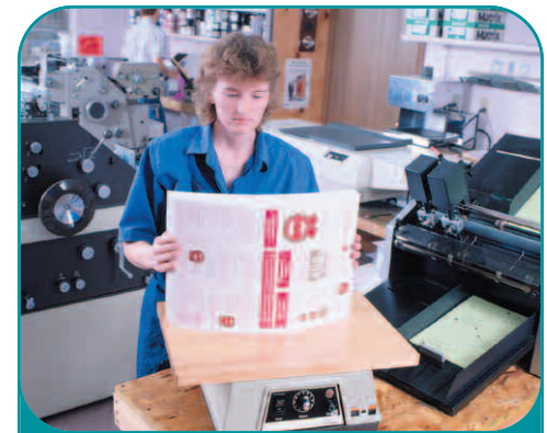
The J-50 jogger aligns papers prior to the folding, cutting or binding process.
