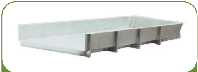
Diagonal Discharge troughs are used to spread the material discharge over the width of a belt or bucket lift positioned at 90 degrees.
