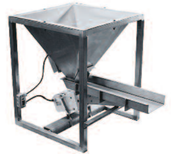
Custom designed FM-152-3 feeder machine with rectangular supply hopper.
