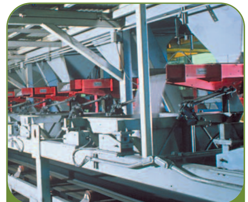
Ideal for controlling bulk material in mixing, blending, batching, grinding and packaging operations, the ten standard Light Industry Electromagnetic Vibrating Feeder models operate with maximum capacities ranging from 1,250 pounds to 25 tons per hour, based on material weighing 100 pounds per cubic foot.
