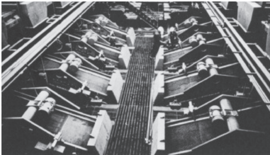
Eight Syntron Model RVS-1512-K vibrating screens equipped with 14-mesh slotted cloth, each producing 25 to 30 TPH of minus 14-mesh fireclay with shale.
