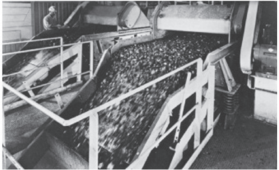
Two Link-Belt® Model SG2616 straightline vibrating screens washing and sizing coal.
