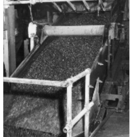
Model UP-2410 handling limestone in a sizing operation at crushing plant.
