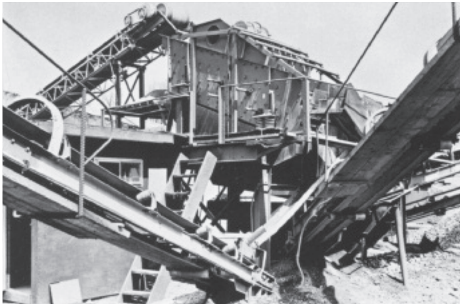
Three-deck Syntron Model RVS-3412-H vibrating screen handling 135 TPH of stone and sand, washing with sprays.
