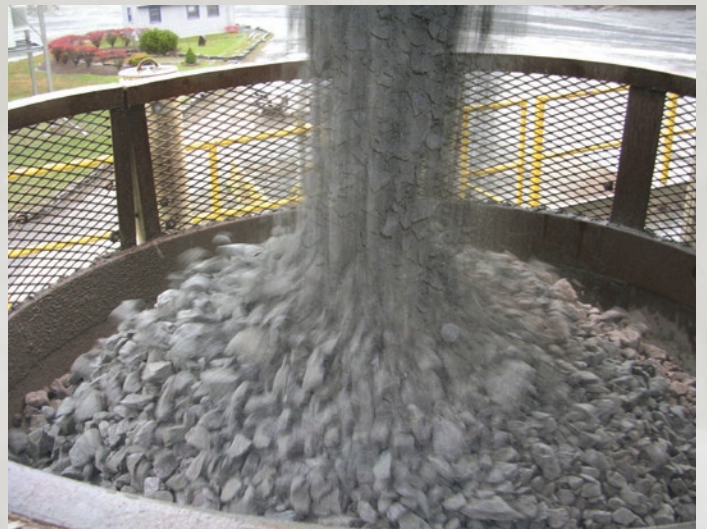
Uniform distribution of material to the cone.
