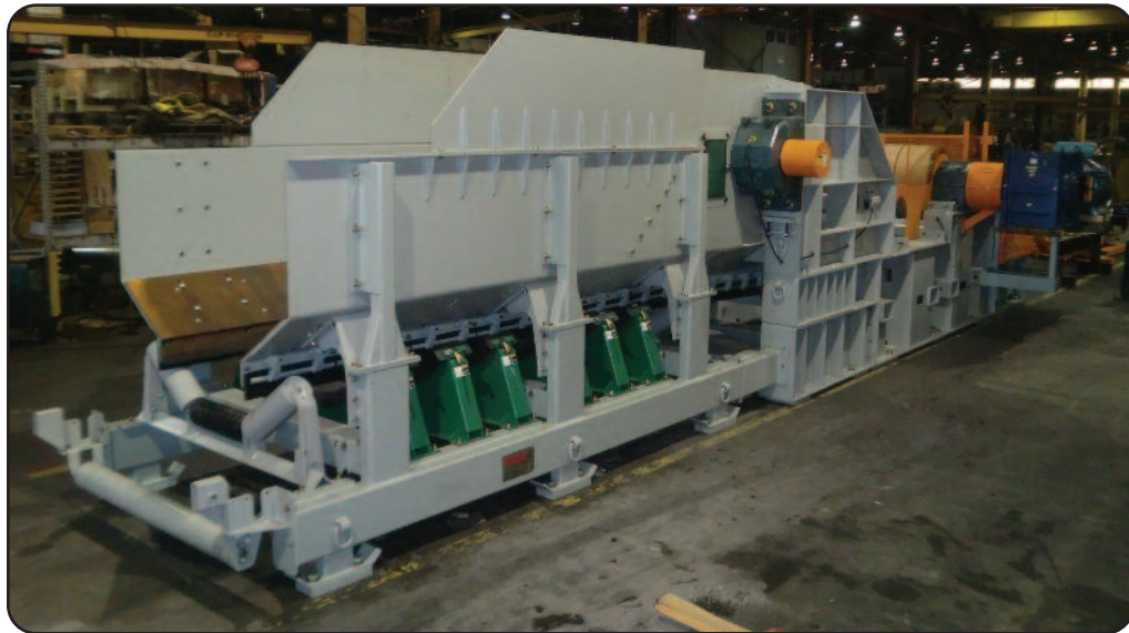
3x500HP Booster/Tripper Drive
